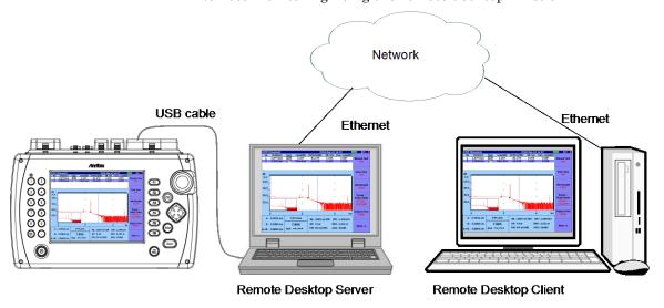
Figure 1.1-2 Example of Remote Monitoring Using Remote Desktop
